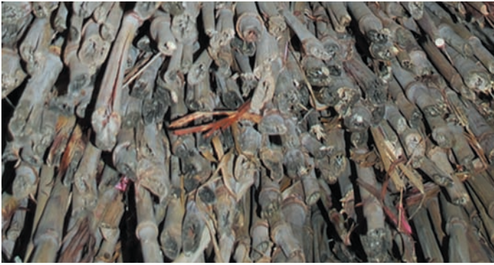
The sorghum stalk has a soft center surrounded by a strong, hard outer ring. By adjusting the pressure applied in forming the stalks into boards, the density of the finished product can be varied.
